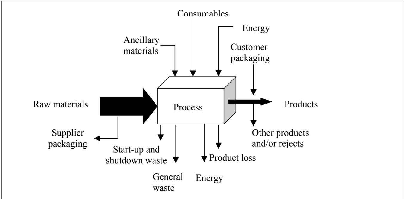
**Figure 2. Material flows through a manufacturing process**
