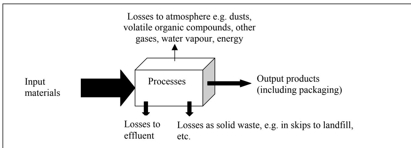
**Figure 1. Generalised process model**
