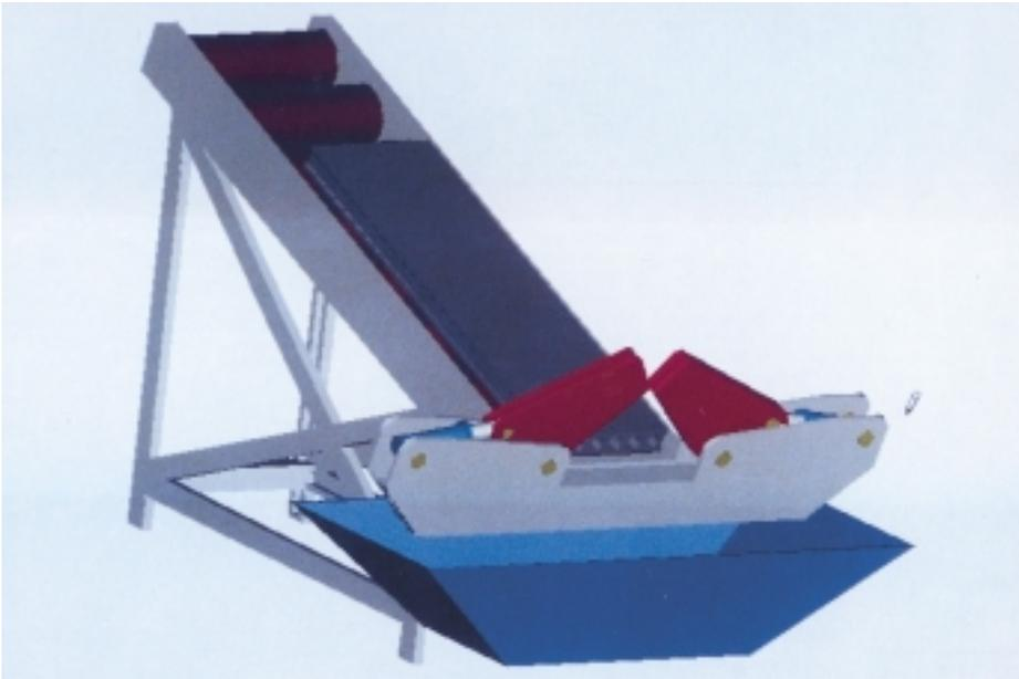
The objective of this project was to design a crusher that combined the necessary technologies that would produce separation of concrete and steel from hollow core concrete safely, efficiently and cost effectively. In addition to the crusher being designed, the environmental benefits of the use of the crusher were evaluated and the economic feasibility of the crusher established.
