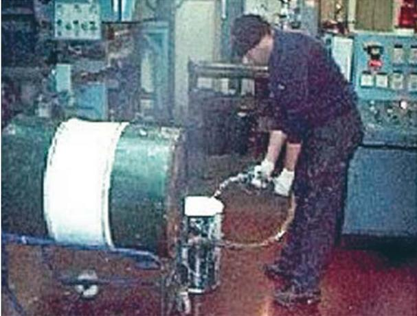
Figure 3: Dispensing solvent from sealed drum
