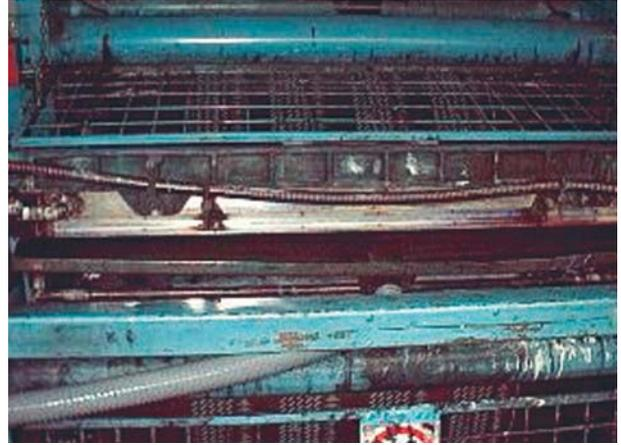
Figure 5: After: tray now empty as ink is pumped directly to reservoir.
