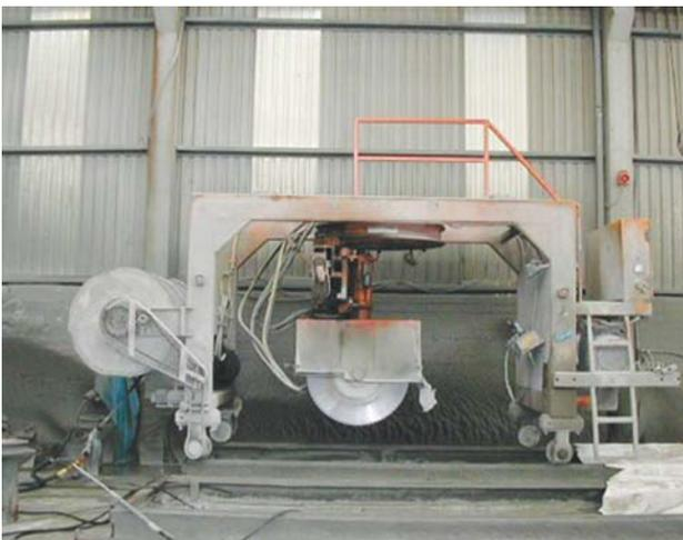
Fig 3. Saw used to cut slabs.
