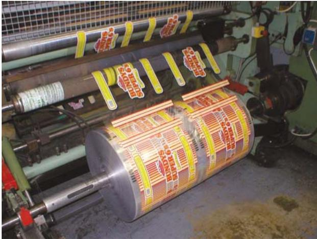
Fig 4. Printed wrap in the process of being slit.
